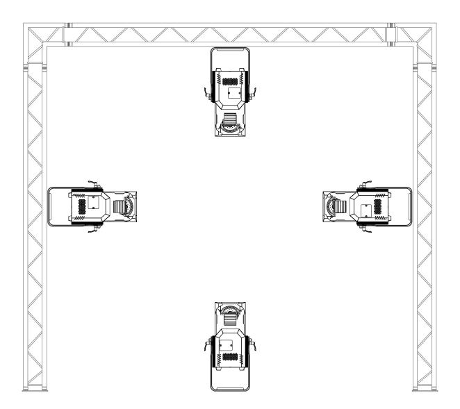
The Helix Roller XP 150W Barrel can be operated in a number of mounting positions as shown in the diagram above, hanging upside-down from the ceiling or truss, mounting sideways on truss or stood upright on a flat level surface. Always use a safety wire as an extra safety precaution to prevent damage/injury in the event a clamp fails (see the next page for clamp installation). Never use the carry handles for secondary attachments.
