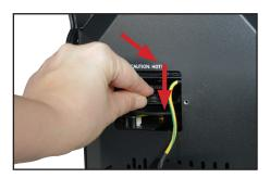
5) Push the gobo holder back into the slot in the gobo wheel and push towards to gobo wheel to ensure it is seated correctly.
