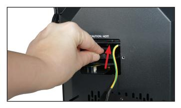
3) Carefully push the gobo holder you are wanting to replace upwards, away from the gobo wheel.
