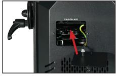
6) Move the gobo access door back into position over the gobo access slot, ensuring the earth wire isn't obstructing any mechanisms.
