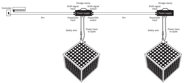
Installation example 2 - For instance if using 1 qube on one zone the maximum cable length between qube power supply and controller must not exceed 18m.
